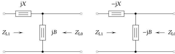
$$W = \frac{Z_{L0}}{Z_{L1}} \quad X = Z_{L1} \sqrt{W - 1} \quad B = \frac{\sqrt{W - 1}}{W Z_{L1}}$$
