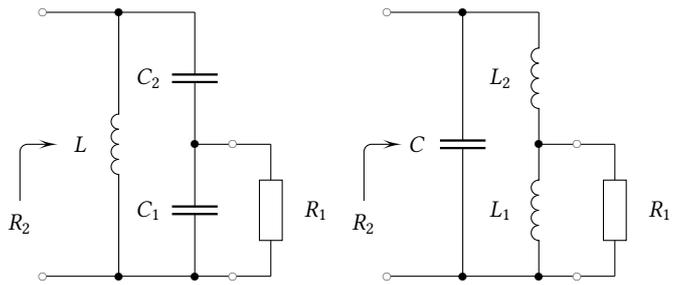
$$R_2 = \left( \frac{C_1 + C_2}{C_2} \right)^2 R_1$$
