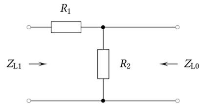
$$\frac{a_{\min}}{\text{dB}} = 10 \lg \left\{ \frac{2 \left( Z_{L1} + \sqrt{Z_{L1}^2 - Z_{L1} Z_{L0}} \right) - Z_{L0}}{Z_{L0}} \right\}$$
